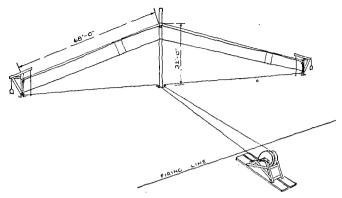
FIGURE 39.-Double climbing and diving target.
